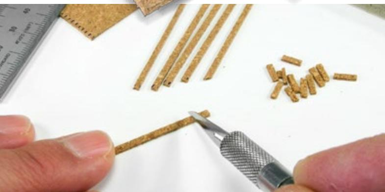
We cut the cork strips 1.5 to 2mm wide and cut the strips into pieces about 7 mm in length until we have enough bricks for our construction.
