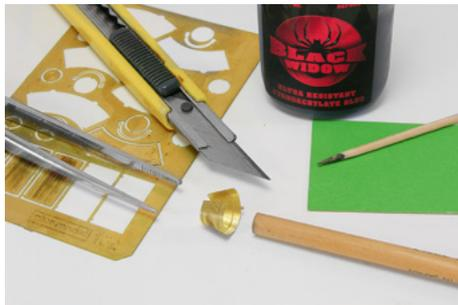
In general we can use cyano to bond almost any type of material to each other. In this example we are going to test the black type in joining photo-etched parts without soldering.
