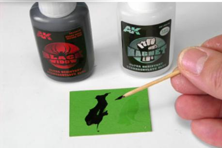
The main difference between the two types is not only their color but also their viscosity, being higher in black cyano. In addition, it dries to a practically matte finish, which facilitates the subsequent painting process.
