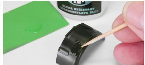
We can also use cyano to create texture on the smooth surface of a piece. This can be useful to simulate the cast finish on some turret or hull parts of an armored vehicle. We apply and distribute it randomly on the piece with the help of a wooden toothpick or another tool.
