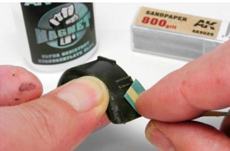
After a few moments, before the glue fully cures, we sand the surface with a medium grit sandpaper, mixing the sanding residue with the fresh cyano. After a few instants and without waiting for it to dry completely, we apply a medium grit sandpaper so that it dries and we mix the residue of the sanding with the fresh cyano.
