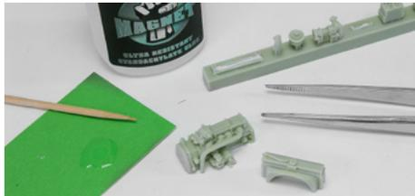
Another of its main applications is connection of resin parts. In this case we will use the transparent type cyano, but the process will be no different: after depositing the adhesive on a piece of cardboard, we use the applicator to apply it to the selected surface of one of the parts to be glued. After mating the parts together using a light pressure, they will be firmly stuck after a few seconds and we can safely continue our work.
