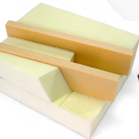
An example of base made from Extruded Foam which was protected with Das Pronto modeling clay that allows for further work on its surface without any problem.
