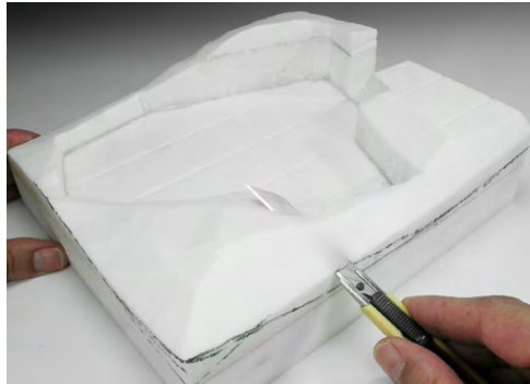
It can be easily shaped. You can also join different pieces with white glue.
