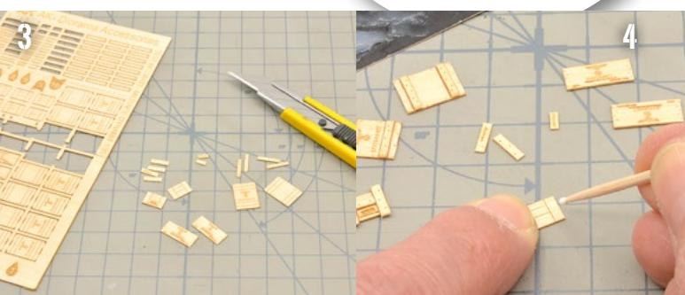
4. For gluing we will use PVA glue that we can apply with the help of a toothpick or pin. The PVA glue allows us to assemble more nimbly and without waiting due to its fast drying speed.
