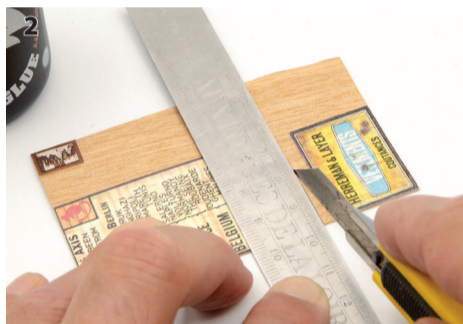
2. The first step is to cut the printed paper and glue it to the wooden board with white glue or double-sided adhesive tape.
