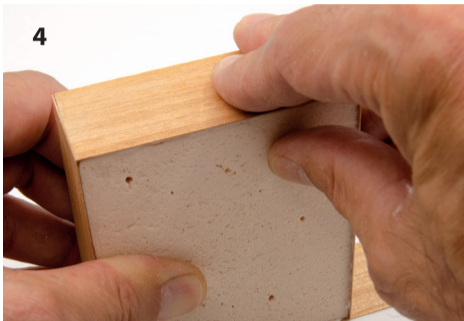
3 and 4. After cutting the piece of wood, apply the glue, position the piece well and apply pressure with your fingers. We will eliminate the excess of glue with a cloth or piece of paper.
