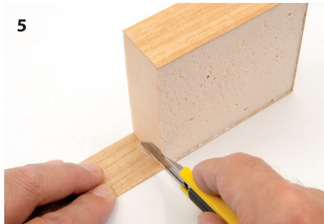
5. Once the glue has dried completely, remove the excess wood with the knife, making sure that a clean cut is left.
