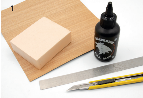
1. The basic working tools are a metal ruler and a sharp knife. To glue it we can use white glue or contact cement, or even cyanoacrylate adhesive. The use of one type of adhesive or another will depend on the work surface since some of them damage materials such as foam or polystyrene.
