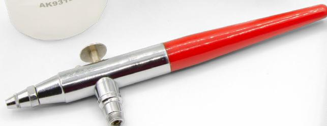
We start by priming the part (Grey Primer AKI1500). We can prime with an airbrush or with a brush. If we use an airbrush we can dilute the primer with a mixture of 35-40% primer and the rest of thinner (or water) and apply it uniformly in layers.
